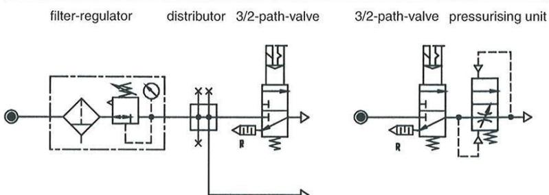
compressed-air plants or parts of plants can be switched on or switched off and ventilated.
